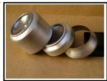
Then position the assembly over the Guinness top, and again, push firmly home. There is no need to crimp, shape or otherwise alter the contours of any of these components. They will fit together like the proverbial glove. The Coke can is fractionally larger than the Guinness can, and this difference allows for smooth assembly.
