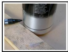
Without the bean tin you will have a runaway burner. The bean tin contains any overfill, and burns it very slowly to assist fuel evaporation within the burner. It is an integral part of the burner design.
