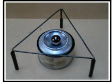
To make the stand, cut a wire coat hanger into three strips and bend them so that each leg is 60mm high. I fit mine together with plastic tube - it doesn't get hot enough to burn. The stand folds flat.
