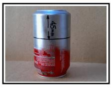
Place the ball-bearing, which should be around 1.5 - 2.0cm diameter, in the centre of the upturned Coke can, and strike it with a hammer to make an indent.
